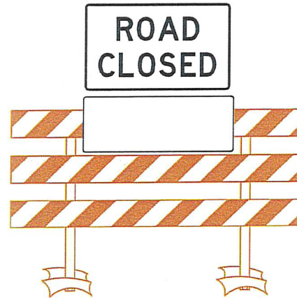
Sign Placement with Supplemental Sign
