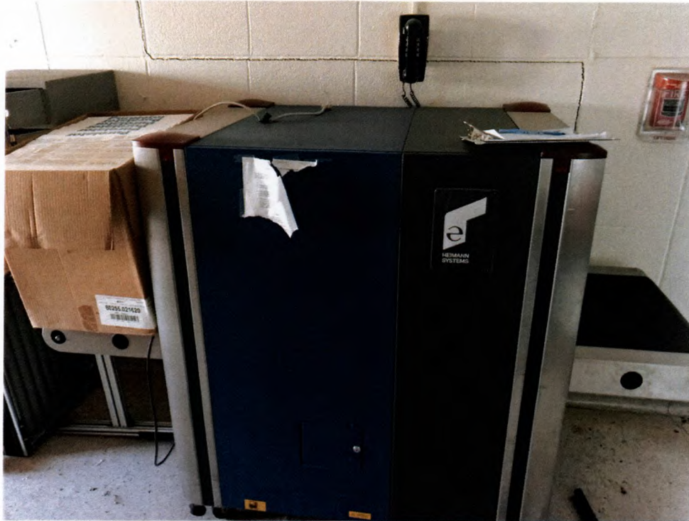
Photograph 19: X-ray inspection unit
