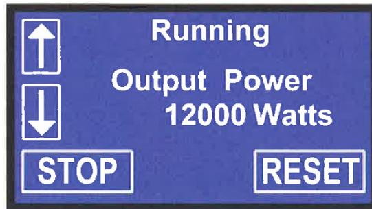
The status of the inverter's operation is shown on the lines one and two of the display. The following table lists the status messages that may appear.
