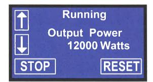
The status of the inverter's operation is shown on the lines one and two of the display. The following table lists the status messages that may appear.
